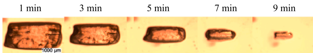
Fig. 1. Shape modification of a sugar grain upon dissolution in water at different times. Adapted from [42].
