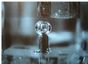
Figure 1: Real (left panel) and schematic (right panel) setup of the experimental apparatus. The central sphere mimics the oscillating bubble.
